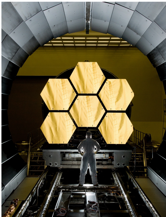
Hexagonal mirror segments of the James Webb Space Telescope under test. NASA/MSFC/David Higginbotham, public domain, via Wikimedia Commons
