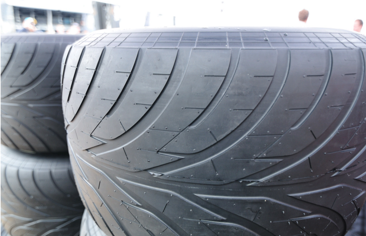
Wet-weather racing tyres showing drainage tread. Gregory Moine, CC BY 2.0, via Wikimedia Commons
