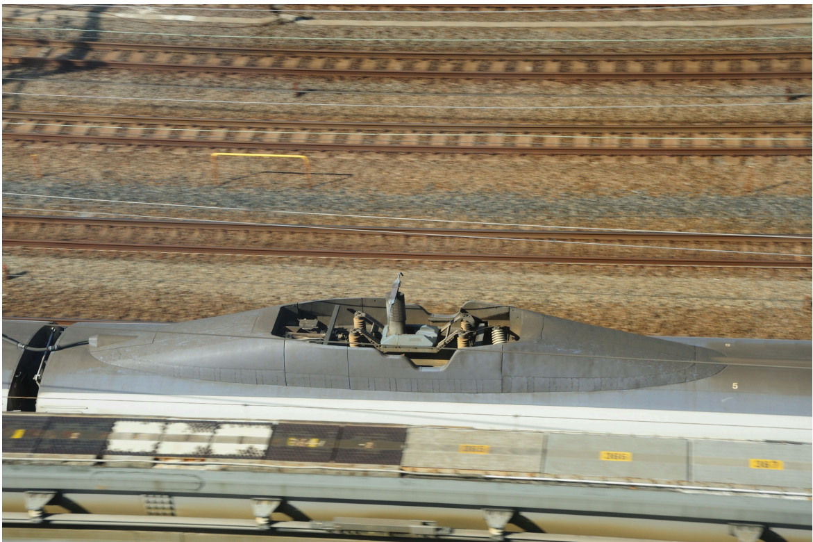
Pantograph and fairing on a 500 Series Shinkansen roof. Takeshi Kuboki, CC BY 2.0, via Wikimedia Commons
